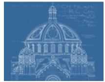
There are several types of prints. Plans are drawn as if looking down at the building. Sections are drawn as if the building were vertically sliced apart along a specific line. Elevations show the vertical surfaces of the building, and detail drawings are larger scale drawings of specific decorative or structural parts.
